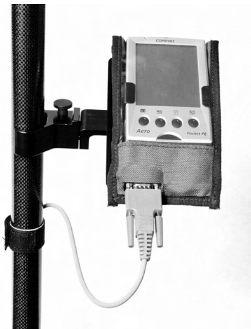
Figure 4.7. Compaq Aero Handheld Mounted on Rover Pole
