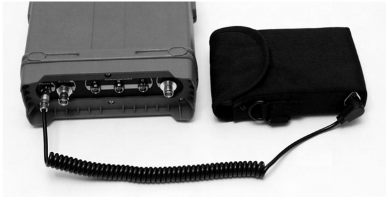
Figure 3.5. Z-Xtreme Connected to External Power
