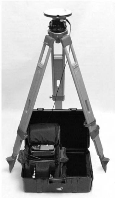
Figure 4.5. Z-Xtreme Survey System Performing a Static Survey
